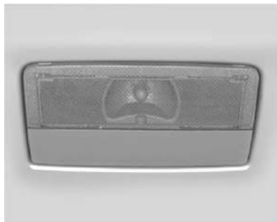
Center Dome Lamp
